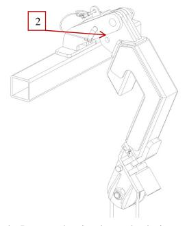
To place in transport mode, Remove the pins, lower the davit arm & re-install the pin (2) & keeper pin to prevent the pins & cables from getting entangled.
