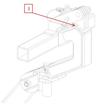
To place in working position, lift swinging davit into the work position & install main pin (1) & keeper pin. The Davit is now ready for use.
