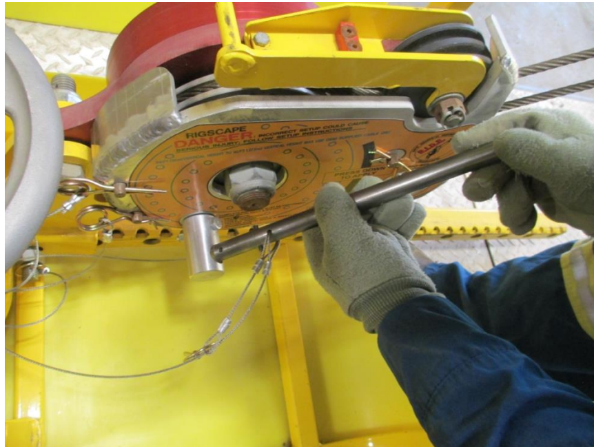
2.1.7. Insert handle into the override-brake hub.
