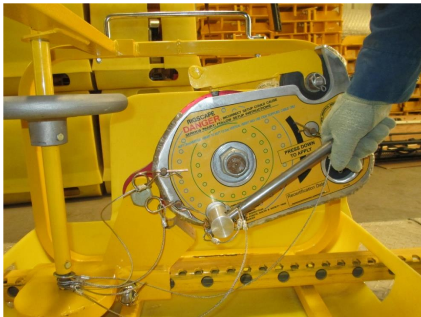
2.1.10. Apply pressure on the handle as in the direction indicated on the Magnegress cover.
