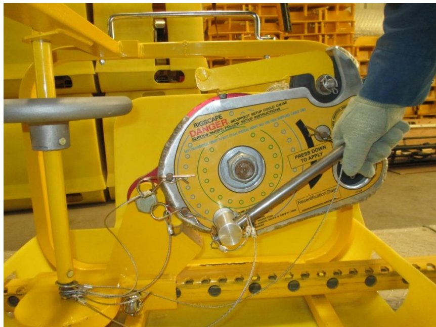
2.9.10 Apply pressure on the handle as in the direction indicated on the Magnegress cover.
