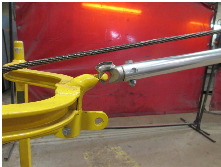
2.12.3.2 Pivot & rotate the Trolley & Spacer Bar assembly.
