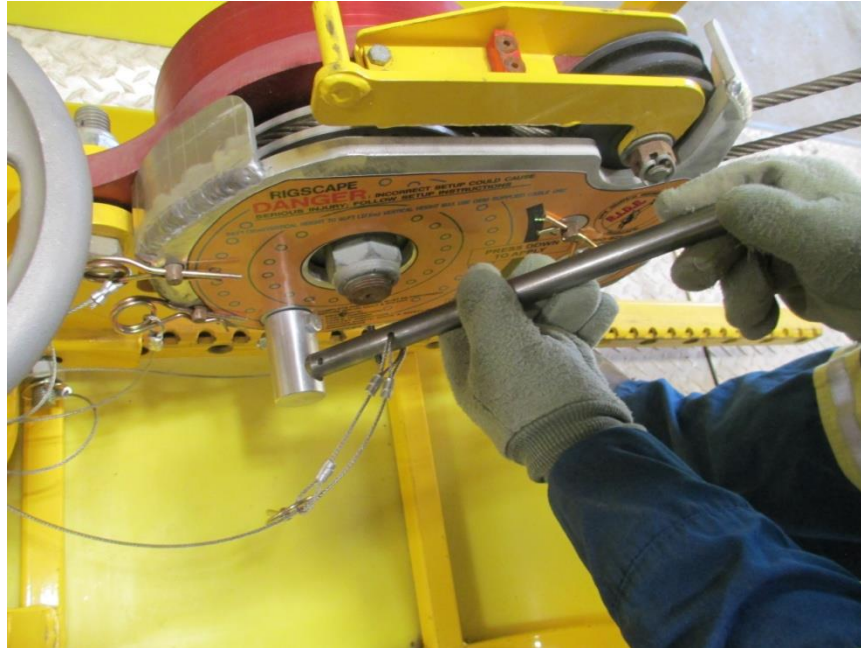
2.9.7 Insert handle into the override-brake hub.
