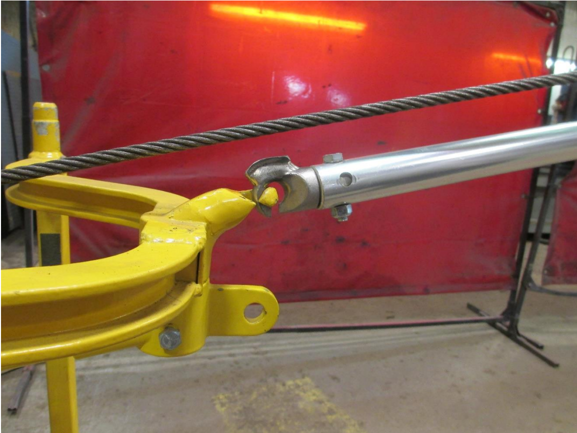
2.12.2.3 Pivot & rotate the Trolley & Spacer Bar assembly.
