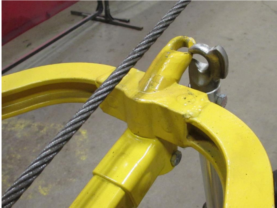
2.12.3.1 Intersect the two ends through the open slots.
