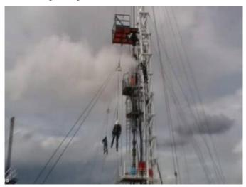
3.1.4. If the worker uses the overhead fall-arrest, his weight will disengage the trolley from the docking station.
