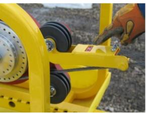
2.8.2. Turn the pinion hand wheel clock-wise, move the brake assembly towards anchor there by tightening the cable, tighten until the indicator pad becomes flush with the top face of the tension indicator. When the two hole line up, insert the adjustment bolt, install the nut and safety pin.
