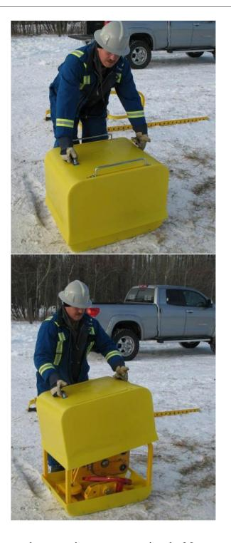
2.4.4. Remove the protective cover, exposing the Magnegress system.
