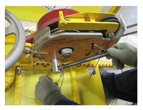
2.9.8. Insert safety pin into the back side of the handle.
