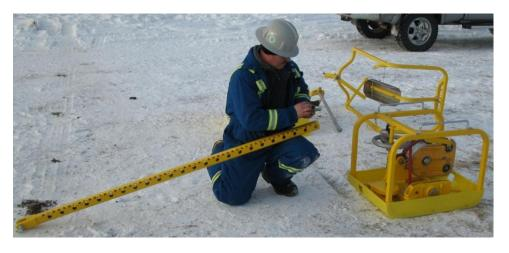
2.4.5. Remove the long adjustment bolt from the receiver tube on the Magnegress frame & the short stopper bolt from the tension link.
