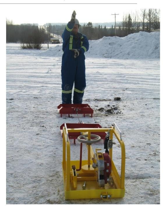
2.5.4. Align the Magnegress system to the top anchor point.
