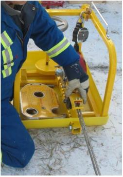
2.8.1. Rotate out the tension indicator. Side slip the cable across the back stop pin until the cable slips to the top of the back stop pin.
