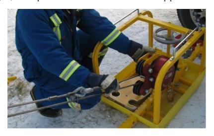
2.8.4. Rotate the tension indicator back into the stored position.
