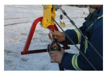
2.11.2. Attach the SRL (Self-Retracting Lanyard) into the SRL anchor point at the end of the tri-handle shank.
