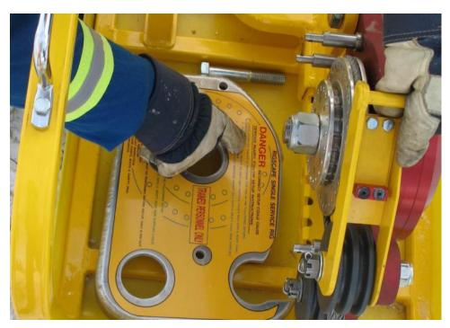
2.7.4. Install the cable on the proper sized sheave as per cover plate decal.
