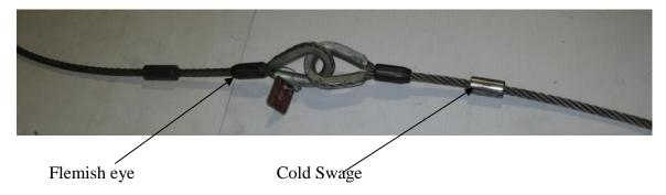
2.2.1. Inspect the cable for frays, kinks or any other damage. Check the Flemish eyes & cold swages for damage or wear.
