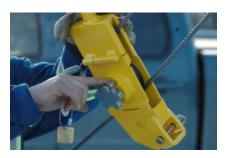
2.10.4. Close the sheave gate & tighten the sheave gate knob clockwise until snug. Turn the lock-pin knob until it drops into the lock position (DO NOT use wrenches to tighten). Inspect the sheave gate's locator flap for damage & for proper fit.
