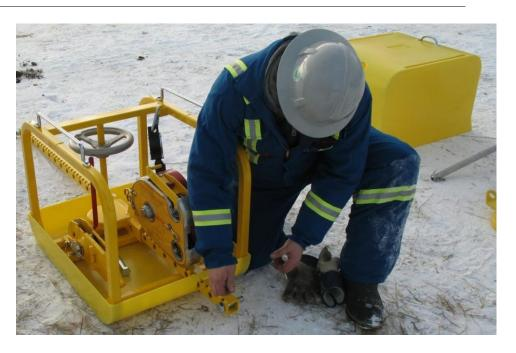
2.4.7. Insert the stopper bolt, nut & safety pin.
