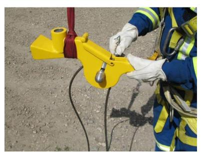
2.3.1.11. Flip down the sheave gate into its closed position & install the safety pin.
