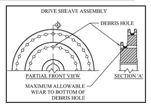
2.7.5. Check the drive sheave debris holes for debris &/or wear.
