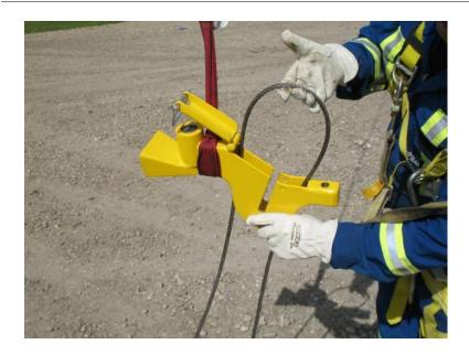
2.3.1.8. Create a 180° return bend on cable and push it through the underside of the Snubscape docking station until the 180° return bend is exposed about 6" through the sheave gate opening.
