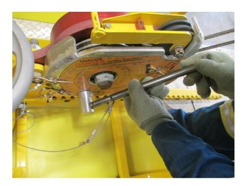
2.9.7. Insert handle into the override-brake hub.
