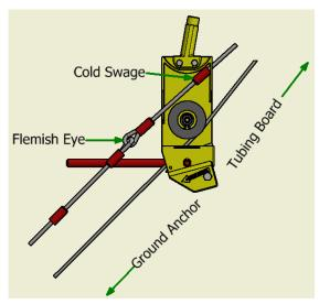
2.10.3. Place the cold swage, located on the upside or tubing board side of the Flemish eye, inside the trolley, above the sheave. Insert the lower cable inside the trolley as well but underneath the sheave. (arrow points towards Magnegress).
