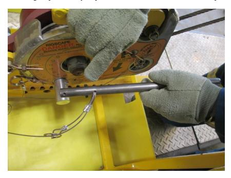
2.9.6. Check to see that the spring pin is properly inserted into the override-brake handle.
