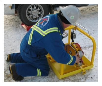
2.7.1. Remove the sheave cover plate from Magnegress brake housing.
