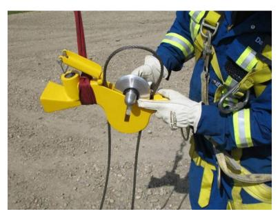
2.3.1.9. Insert sheave inside the  $180^{\circ}$  back bend & line up the flats on the sheave shaft to the slots in the docking system.
