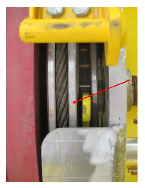
2.9.11. The override brake pad (arrow) should ride the center of the outer sheave.
