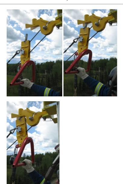
2.11.2.2. Guide the docking pin on the trolley housing into the docking station's receiver tube.
