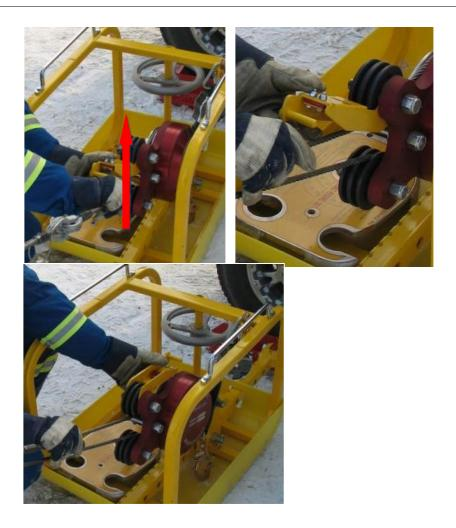
2.8.3. Again, side-slip the tensioned cable off of the back stop pin.
