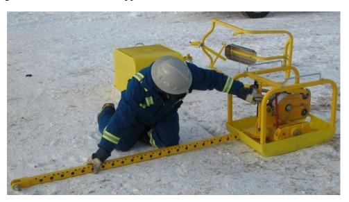
2.4.6. Install the tension link into the receiver tube from the back side of the Magnegress. Turn the pinion hand wheel clockwise to draw the tension link into the receiver tube until the stopper bolt hole is fully exposed on the front side of the receiver tube.
