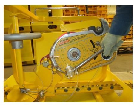
2.9.10. Apply pressure on the handle as in the direction indicated on the Magnegress cover.
