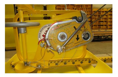
2.9.9. This is a view of the assembled override-brake with handle installed.
