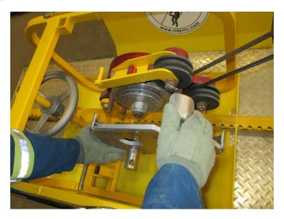
2.9.3. Place the cover onto the Magnegress brake system.
