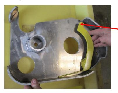
2.9.2. With the cover off check that the brake pad moves freely & that the spring returns the pad to its resting position against the back plate of the cover (arrow).
