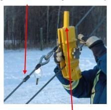
2.10.5. Check the docking pin for debris or damage.
