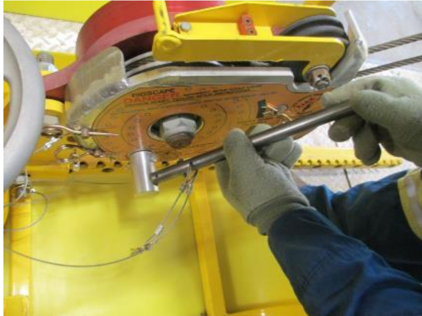
4.10.7. Insert handle into the override-brake hub.
