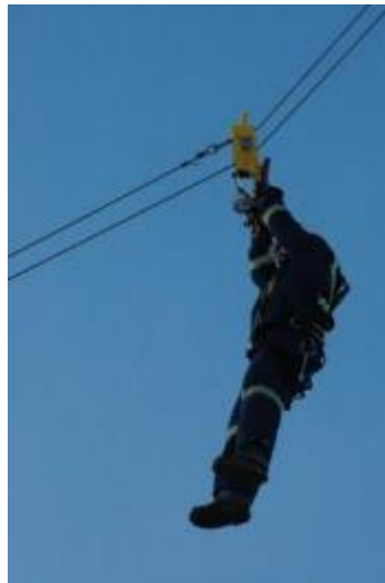
2.15.1.2. Applying weight to the tri-handle releases the trolley from the docking station. The Magnegress brake will automatically control your descent.
