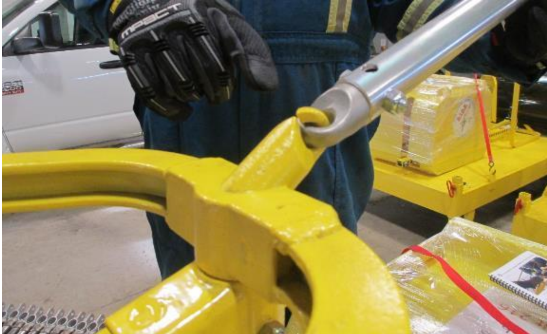
3.13.3. Pivot & rotate the Trolley & Spacer Bar assembly.
