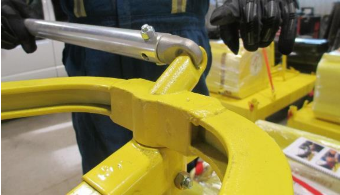
4.12.3. Intersect the two ends through the open slots.
