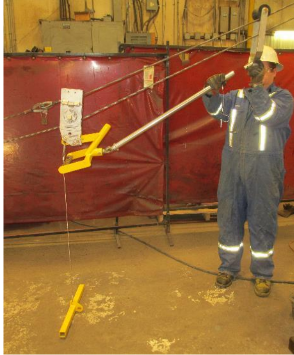
3.13.5. Connect the spacer bar to the fall arrest trolley
