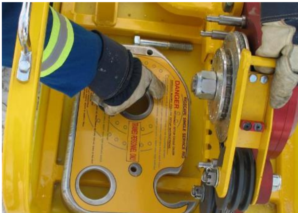
3.8.4. Install the cable on the proper sized sheave as per cover plate decal.
