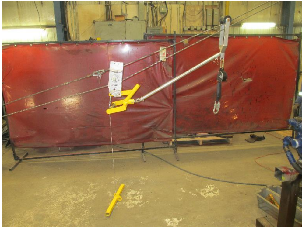
3.13.6. Attach the SRL (Self-Retracting Lanyard) into the SRL anchor hole of the mount.
